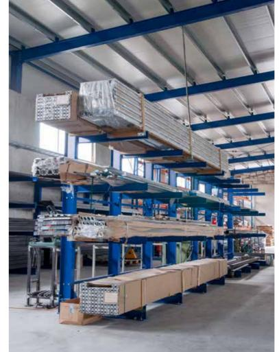
This storage system is so versatile that different component combinations can be used in various situations. The cantilever arms can be easily adjusted in height.
