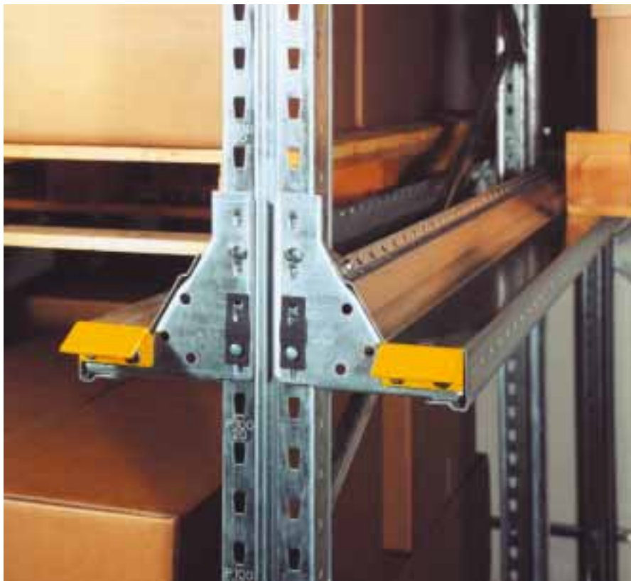
Productivity and safety are increased by the use of high visibility upright guards and guide rails.
