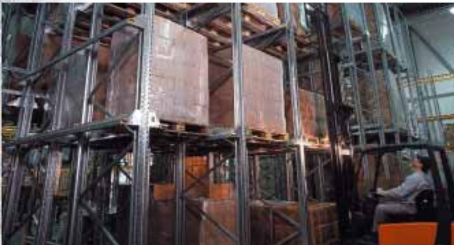
P90 Drive-In racks maximise storage density.
