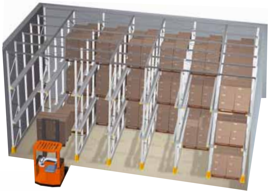
P90 Drive-In racks maximise storage density.
