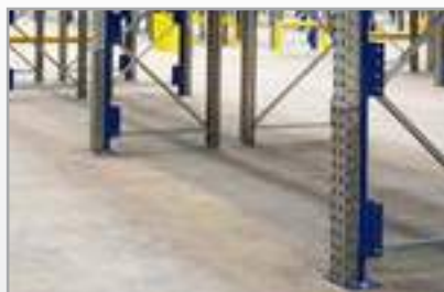
Sacrificial Legs (incl. upright section) - A non-load bearing, removable section of upright, replaceable if damaged, without the need to unload a complete bay.
