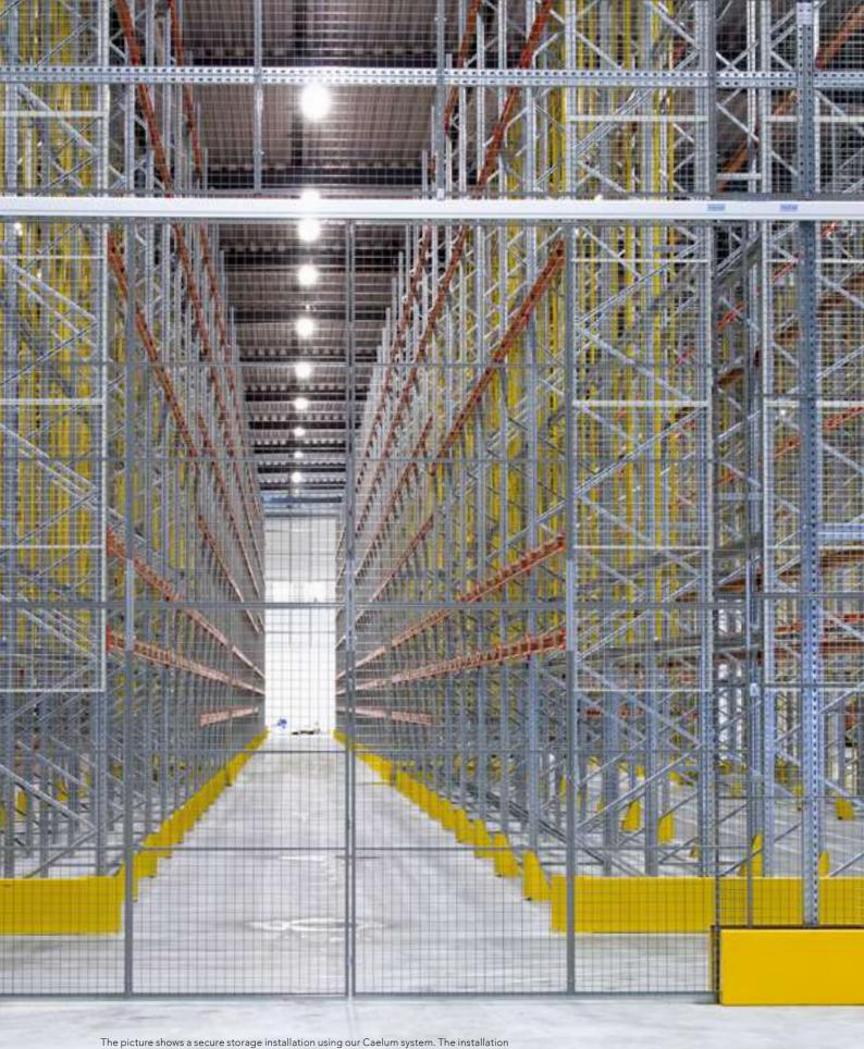
The picture shows a secure storage installation using our Caelum system. The installation required an 11 metre high wall with attachment to the existing racking end frames. A double sliding door in a single rail was also installed for access.
